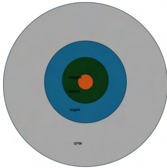
Figure 3: Cell relative area per modulation scheme (illustrative)
